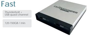
**Dimensions:** 120mm\*100mm\*20mm (Length x Width x Height) Storage Channel Interfaces: Thunderbolt 3 x 2, USB-C x 2 External Interfaces: USB-A (3.1 Gen2, 10Gbps) x 2 Power Input: 12V (18W), supports power supply from power banks and charging adapters
