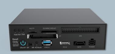
Supported storage media : USB 3.0/2.0/1.0, PCI-E(with PCIe Adapter), SATA, CF/M2/TF/SD/MMC/MS/xD
